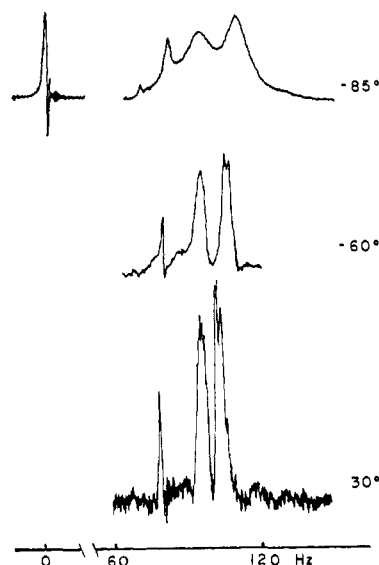
Figure 1. Proton nmr spectra of the ring protons of (\text{CH}_3)_3\text{Sn-C}_5\text{H}_4\text{CH}_3 showing broadening at temperatures below -60^\circ . Note that the benzene resonance (as internal reference) remains sharp at this temperature. The peak at 80 Hz is due to the cyclopentadienyl resonance of (\text{CH}_3)_3\text{SnC}_5\text{H}_5 . (Resonances are given in Hz upfield from benzene.)
